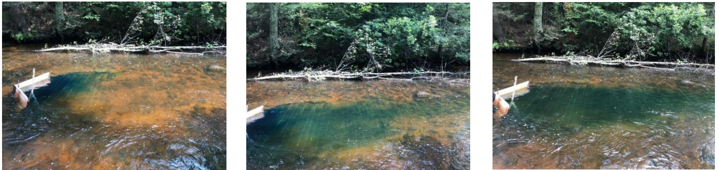
Figure 8. Brilliant Blue dye injected into the groundwater as a tracer showing the development of a groundwater plume over several minutes of pumping.
