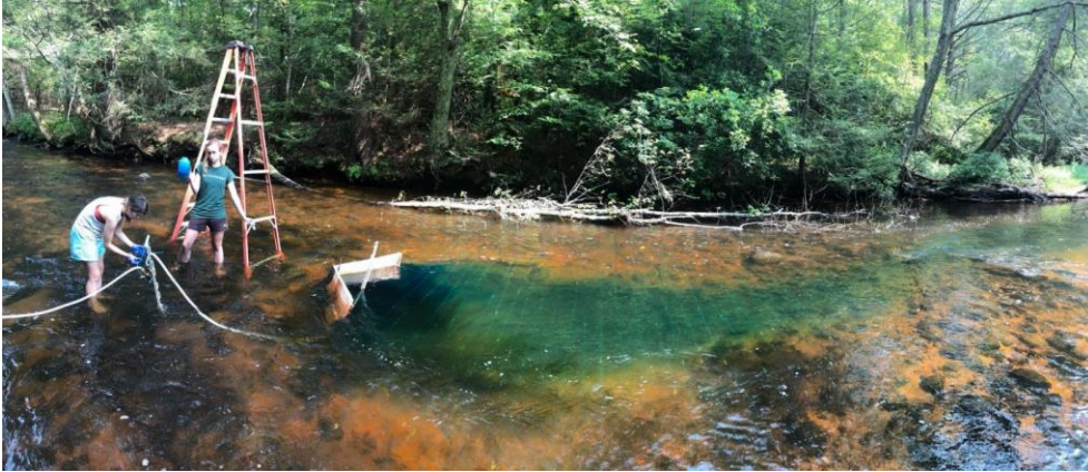
Figure 7. Brilliant blue dye used as a tracer in groundwater, added to hose line.
