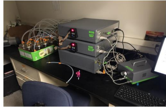
Figure 2. A Picarro gas analyzer and 16-port manifolds were used to quantify CO 2 accumulation rates from forested wetland soil subjected to salinity treatments in incubation jars over a 24-hour period (carbon mineralization).
